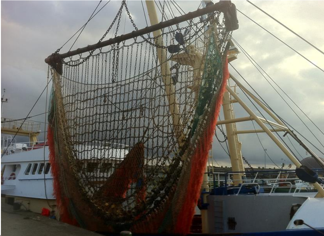
Plate 6.1 Traditional beam trawl with tickler chains and chain mat (Source: BMM, 2012)
