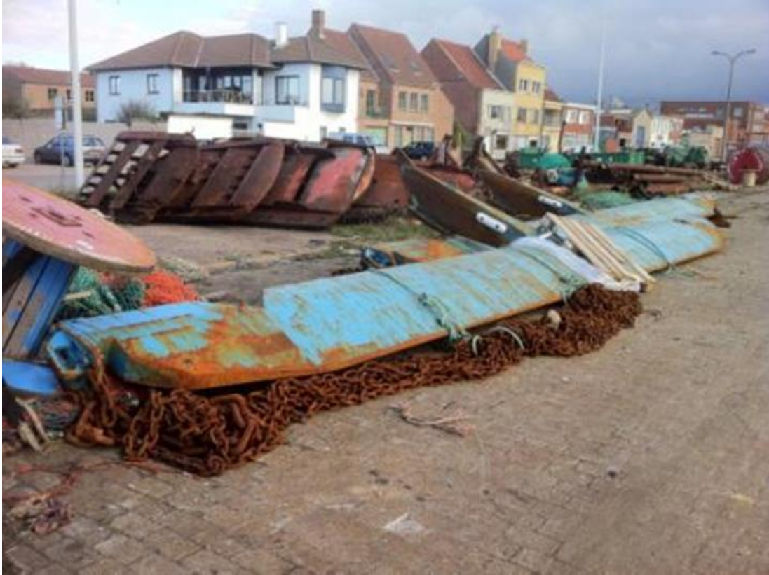
Plate 6.3 Sumwing trawl with attached tickler chains (Source: BMM, 2015)
